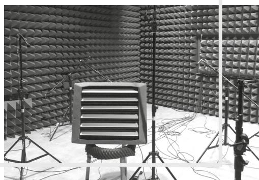
test of accoustic pressure level
