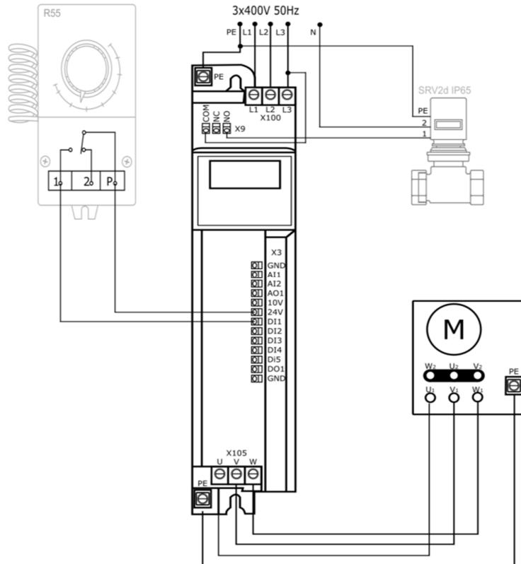
Connection of the R55 thermostat to the inverter, on / off control of the fan and valve actuator as a function of temperature.
