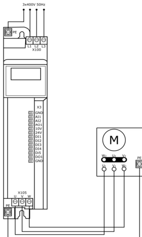
Inverter- (FAL 0.75 3x400) enables stepless adjustment of fan speed using a signal from the microclimate computer (not provided by FLOWAIR). The inverter has the ability to connect the thermal protection of the fan and change fan rotation LEFT / RIGHT.
