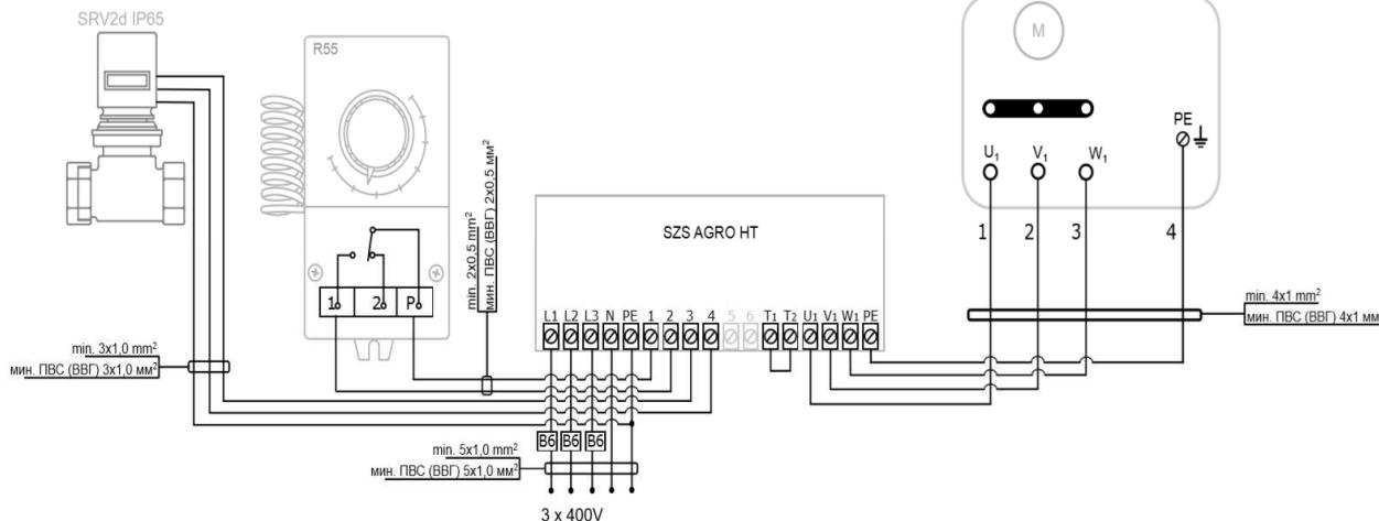
R55 thermostat controls the valve (SRV2d IP65 - optional) and the fan. SZS AGRO HT Cabinet indicates the operating status or failures, controls the phase order, phase asymmetry and phase loss. The cabinet is equipped with a function to change the fan rotation (LEFT / RIGHT). Wires size and type should be chosen by the designer.
