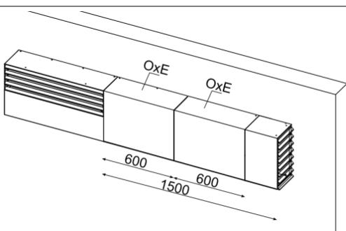
OxE – extension for OxS. It allows to dismiss air intake from air exhaust.
