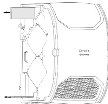
The condition of filter is controlled by pressure transducer. When the filters are too heavily soiled, an alarm is displayed on the T-box controller screen. In this case, replace the filters is necessary.
