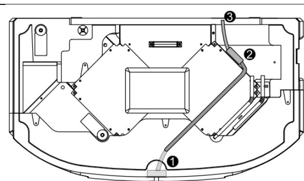
During ventilation and heat recovery process condensate can appear, condensate pump remove it automatically by outlet on the top side of unit.
