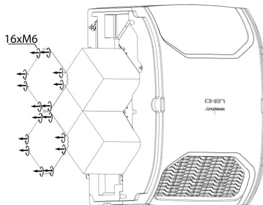
Heat recovery exchanger should be cleaned with pressured air along lamellas.
