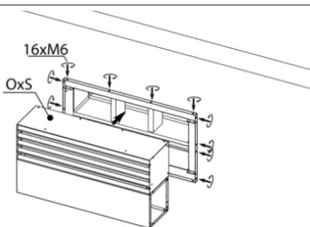
OxS should be installed on the frame already.
